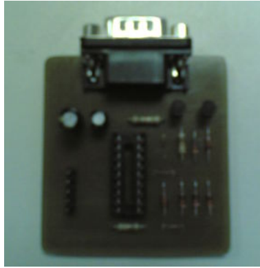
Fig. 6. JDM programmer circuit
